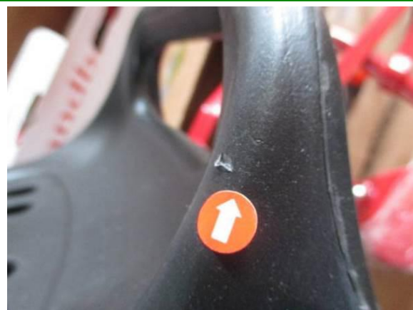
69). Major defect – plastic flash on seat(not sharp)
