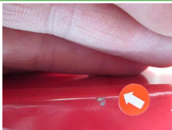
75). Minor defect – paint peeled off on bucket
