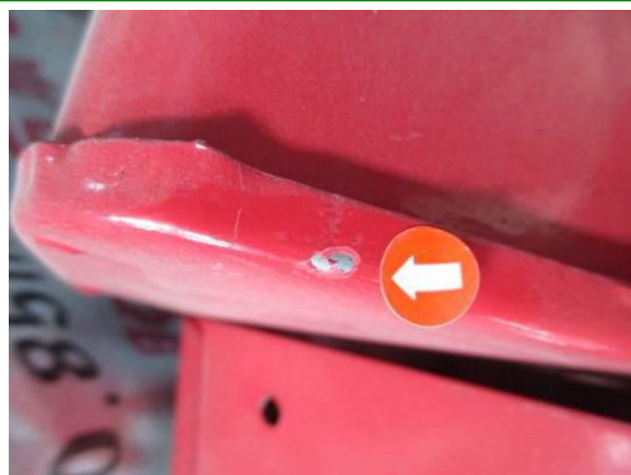
77). Minor defect – paint peeled off on bucket
