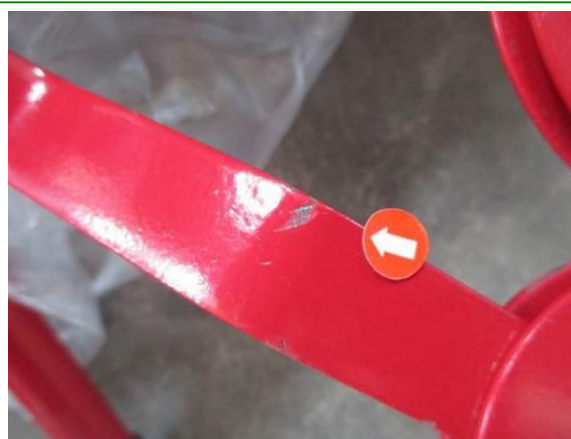
74). Minor defect – paint peeled off on frame
