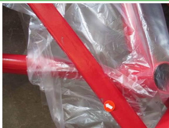
73). Minor defect – paint peeled off on frame
