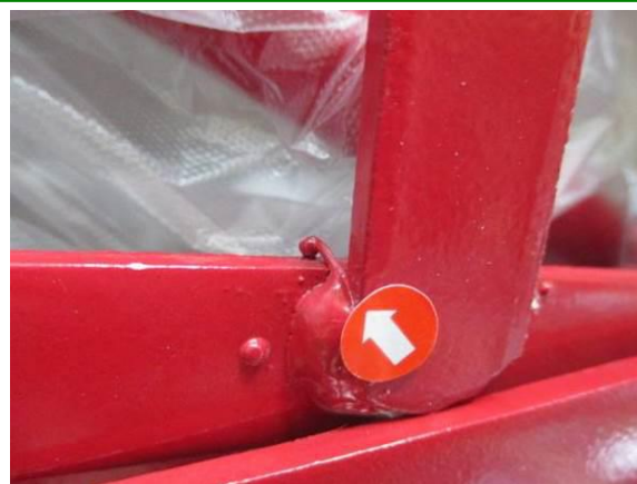
70). Minor defect – slag attached on body
