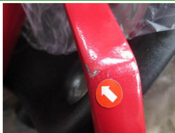
72). Minor defect – paint peeled off on frame
