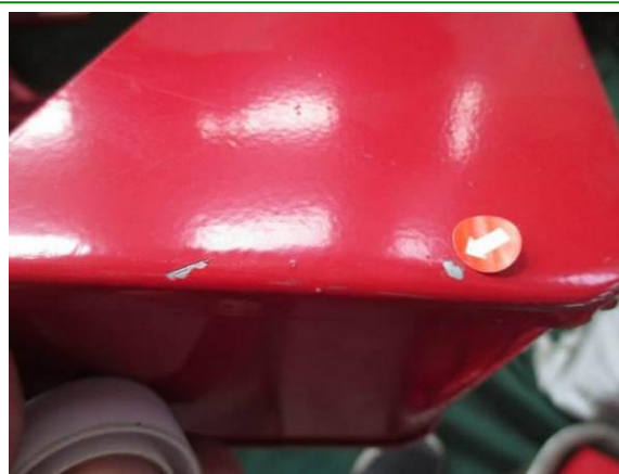
76). Minor defect – paint peeled off on bucket
