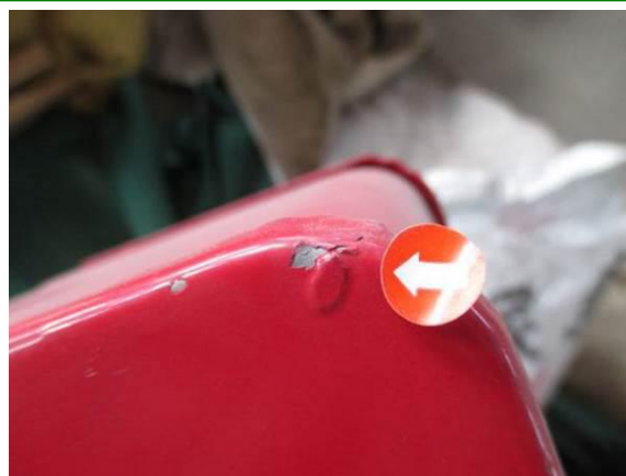
78). Minor defect – paint peeled off on bucket
