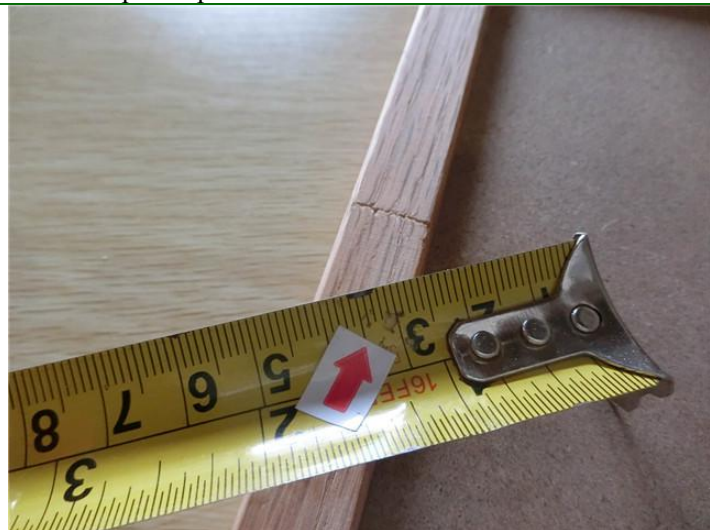
75. Defect: crack on surface --major(total 7pcs)
