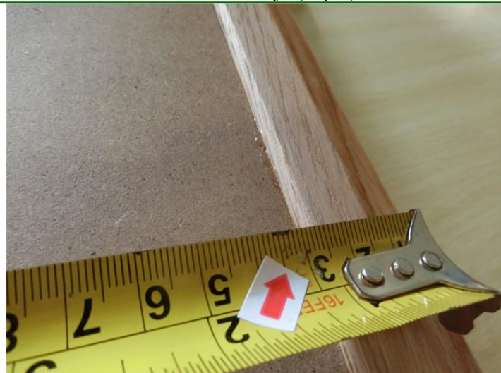
32. Defect: Glue mark --minor(total 26pcs)
