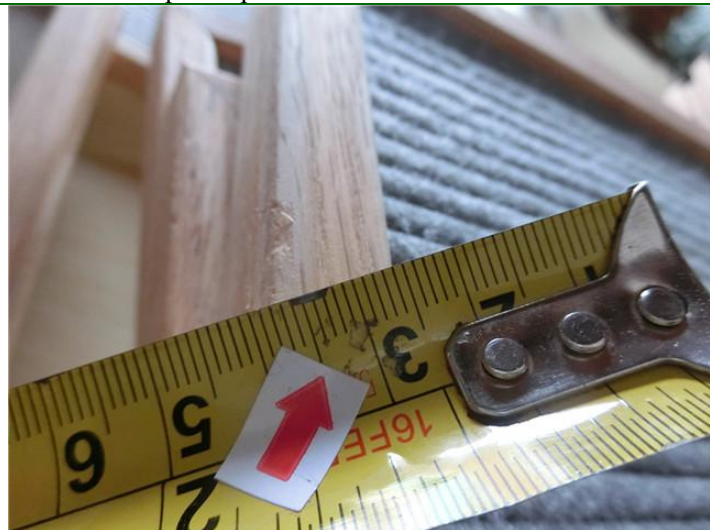
76. Defect: crack on surface --major(total 7pcs)
