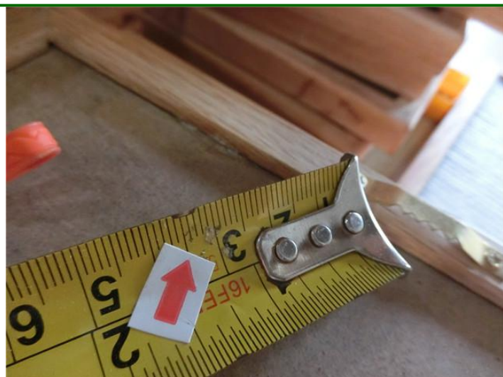
78. Defect: glue mark --minor(total 6pcs)
