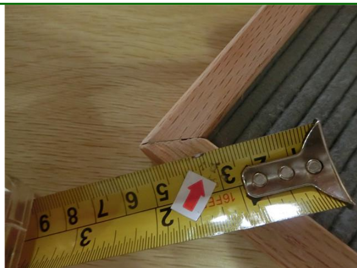
77. Defect: gap on surface--minor(total 1pcs)
