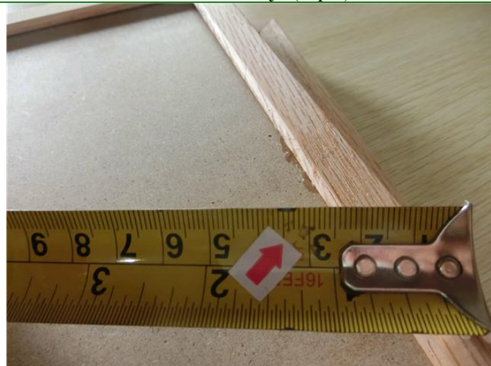
31. Defect: Glue mark --minor(total 26pcs)
