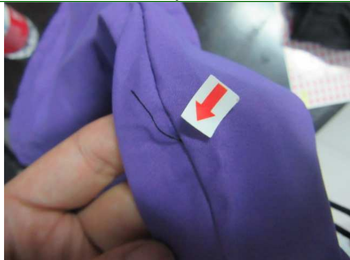
61. Defect- Uncut thread end-minor
