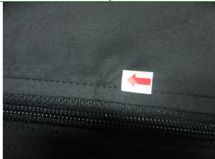
77. Defect- Puckering on top stitch of placket-major
