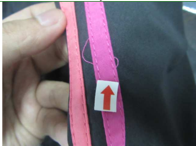
78. Defect- Uncut thread end-minor
