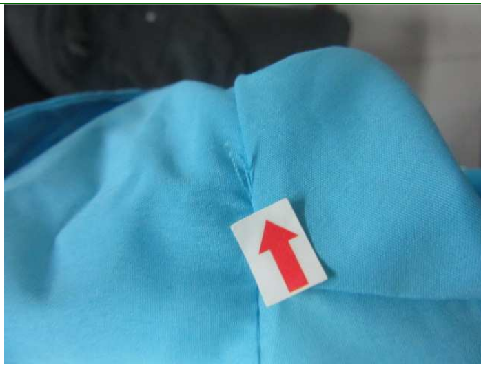
46. Defect- Uncut thread end-minor
