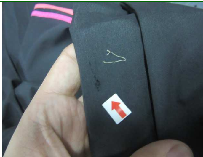
80. Defect- Unclean thread on surface-minor
