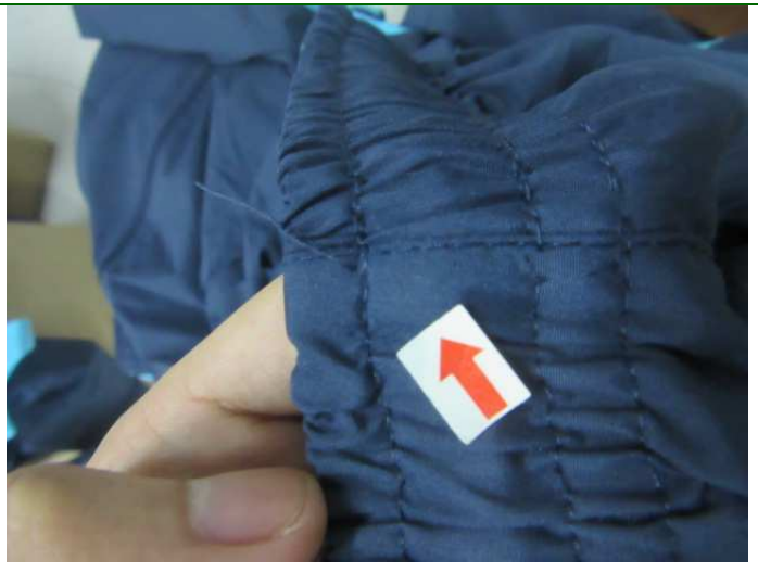
48. Defect- Uncut thread end-minor
