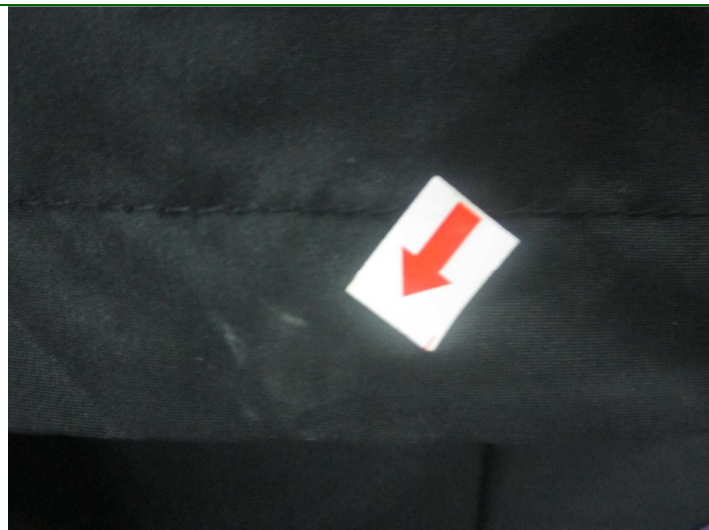
45. Defect- Dirty mark on bottom of pant-minor
