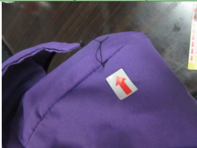
62. Defect- Uncut thread end-minor
