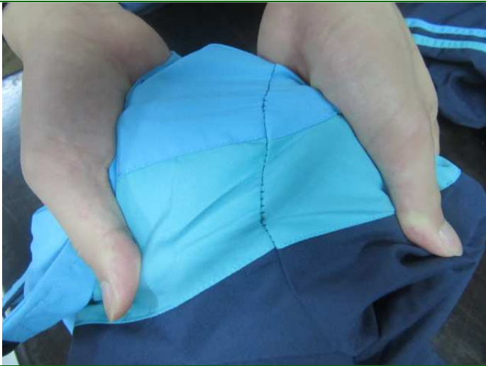
87. Seam strength test
