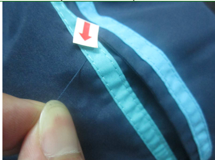
47. Defect- Uncut thread end-minor
