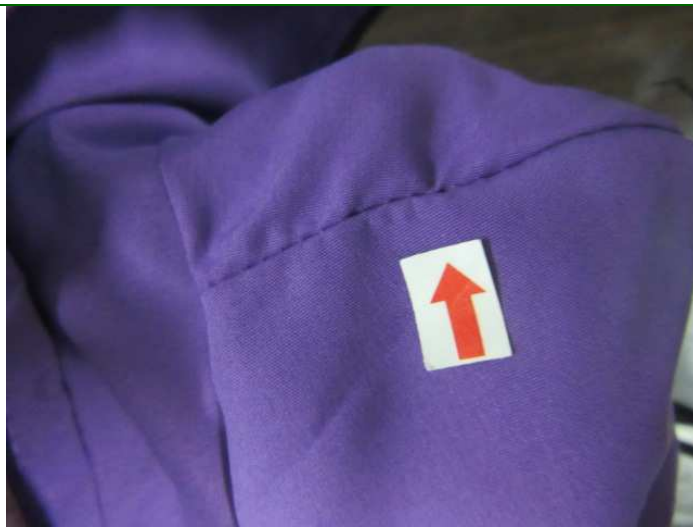
60. Defect- Puckering on armhole seam-major
