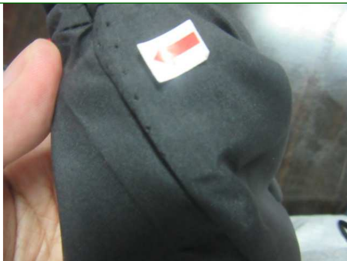
44. Defect- Needle hole mark on pant-major
